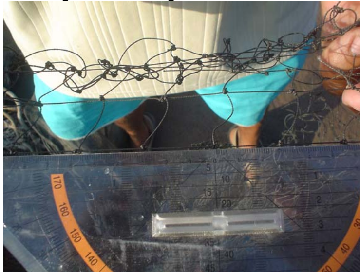
Figure c: Measuring the Fishnet Mesh Size
