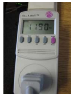
Figure 2. Kill A Watt meter during printer warm up state.
