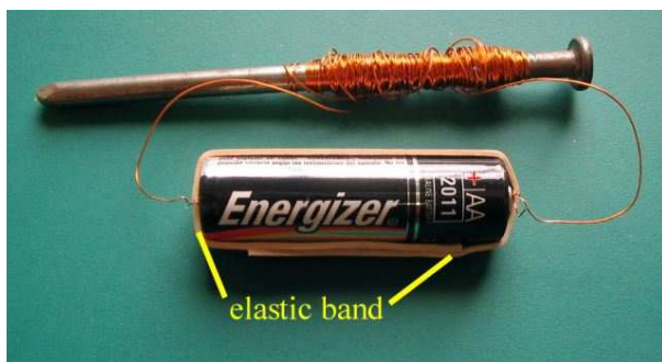
Figure 2: The current carrying copper wire in the above figure creates a magnetic field in the metallic nail.
