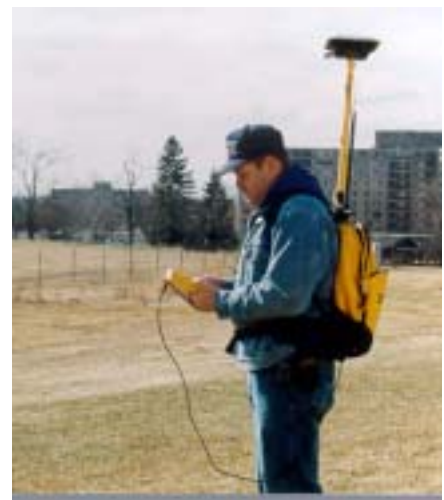
Left, Utilities Documentation Technician Mike Farris displays a GPS receiver that is part of a rover kit. Rover kits are used for accessing data and locating objects that lie below the ground’s surface. Right, Farris uses the rover kit in the field.
