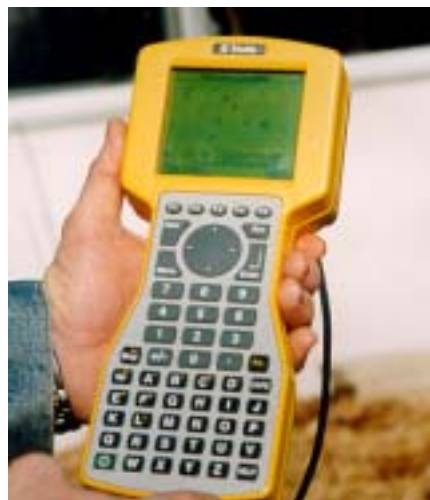
Left, Utilities Documentation Technician Mike Farris displays a GPS receiver that is part of a rover kit. Rover kits are used for accessing data and locating objects that lie below the ground’s surface. Right, Farris uses the rover kit in the field.
