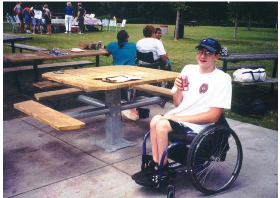
Fixed pedestal square table with one bench removed for wheelchair access.
