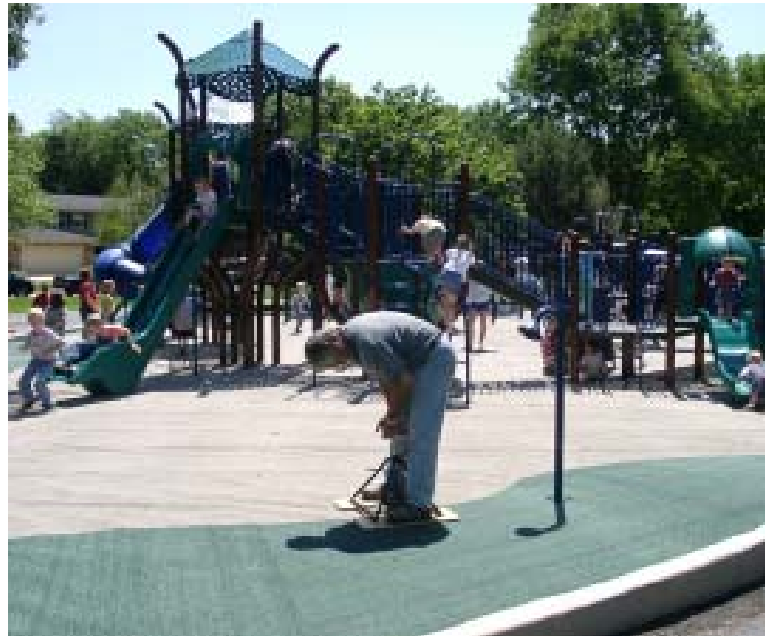
Ken Kutska, Director of the Wheaton (IL) Park District, tests the accessibility of a playground surface with a Rotational Penetrometer as part of the NCA Playground Surface Study.
