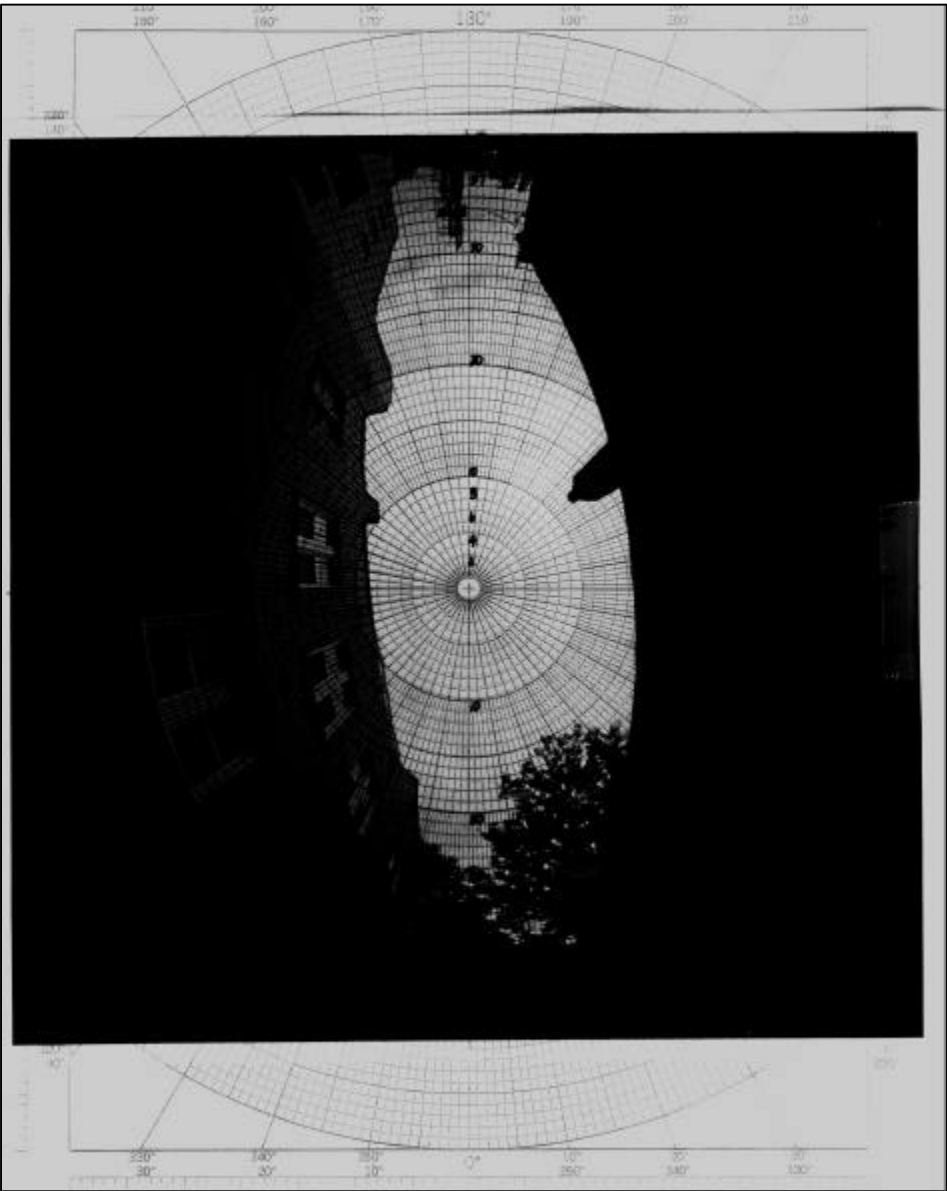
Figure 3. Example of a fisheye photo of an urban canyon placed over polar coordinate graph paper used for the manual analysis
