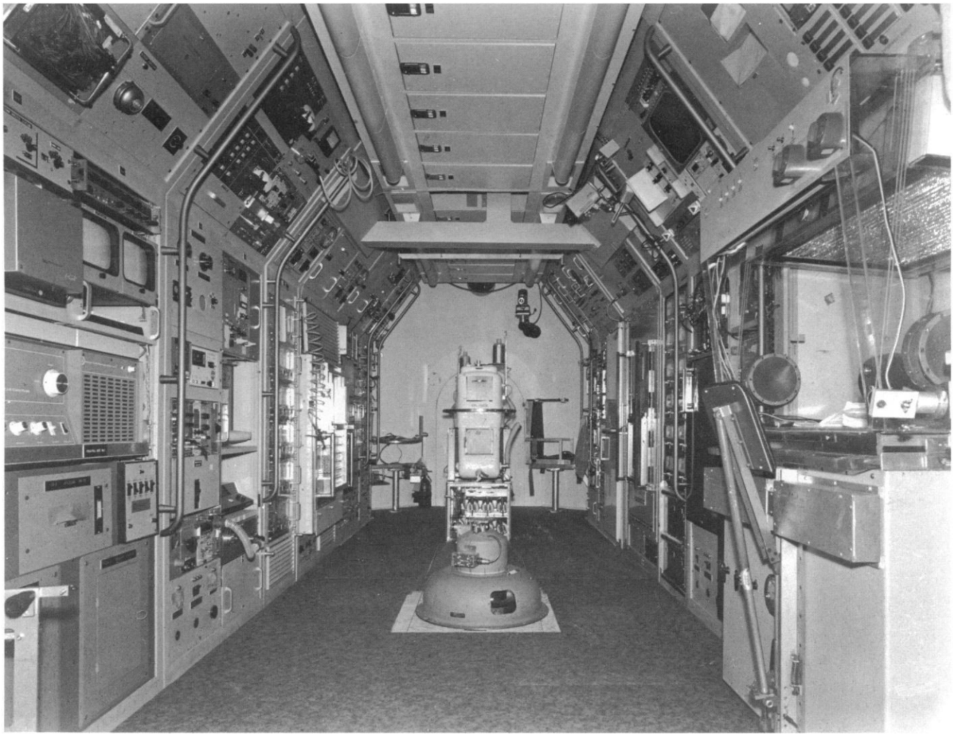
Figure 5. Interior of the European-built Spacelab illustrating the pressurized laboratory module, which flies in the space shuttle's cargo bay.
